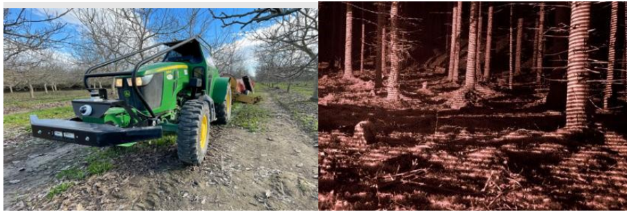
Figure 2: LIDAR sensor mounted on a tractor and a sample point cloud example from this setup (Images taken from https://ouster.com/ ).
