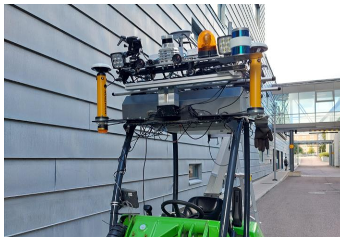
Figure 9: The sensor rig mounted on Avant wheel loader.
